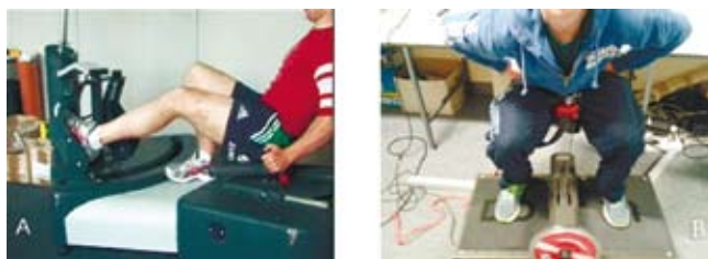
Fig. 2. A) Example of one rugby player resisting to the force exerted by the moving arm (this ergometer was invented by author but it is no longer available on the market. B) One of the commercially available flywheel (the rotating disc in red at the bottom of the picture) equipment allowing to train concentrically and eccentrically
